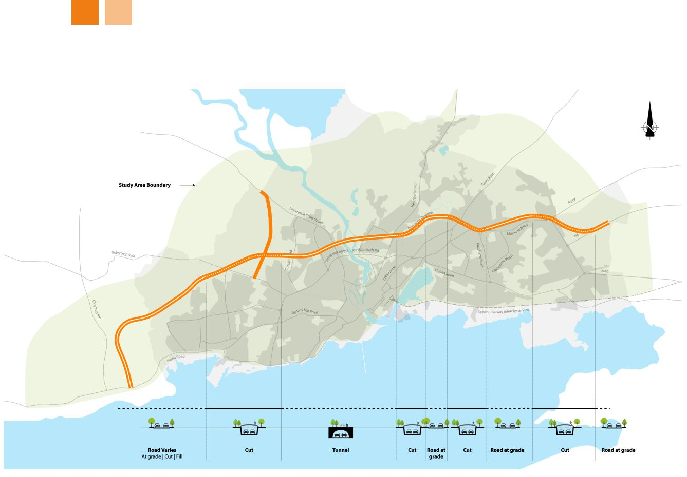
The Orange Option commences at the R336 to the east of Bearna and proceeds northeast to the townland of Na hAille and through Letteragh. From here the Orange Option enters a tunnel, crossing under the River Corrib and emerges from the tunnel at Terryland. The Orange Option joins the existing N6 and follows this road to Coolagh where it terminates at the N6.
